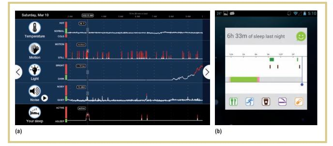
Figure 3. Screenshots from Lullaby and SleepTight: (a) Lullaby's data review screen and (b) SleepTight's data capture widget on Android's lockscreen.
