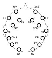
Figure 6: Electrode positions on the headset [2]
